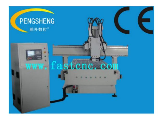
This machine has more completed functions, higher efficiency and more convenient operation mode, mainly applicable in producing plate furniture such as wooden door, cabinet and office furniture, and is based on plate engraving and horizontal drilling and milling. The best advantage of this machine is that It can engrave the key hole in the door easily and conveniencely.
